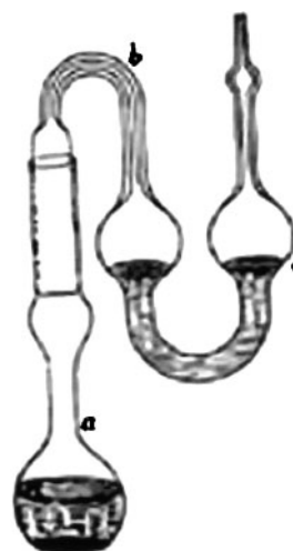
Fig. 5. Apparatus of Fischer & Thierfelder (1894) for measuring sugar fermentations by yeasts; total height about 6 cm. a, Fermentation flask; b, S-trap for CO 2 produced; c, aqueous Ba(OH) 2 . The flask could contain 70 mg sugar in 0.35 ml H 2 O + 0.35 ml aqueous yeast extract + 13 mg of yeast to be tested. Incubations were for 3–10 days at 24–28 °C.
