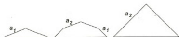
Fig. 8.36. Island shape transitions are represented in Figure 8.35 under the assumption that only abrupt transitions from one conical shape with relatively small aspect ratio a_1 to another with relatively large aspect ratio a_2 are possible. This diagram suggests a more gradual transition from one conical shape to another, effected by having the steeper orientation a_2 gradually expand on the lateral face of the island until the transition is completed.
