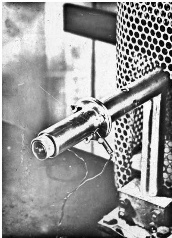
Fig. 2. Prototype model of Ehrenberg-Spear fine-focus X-ray tube used in early muscle work (diameter of tube is approximately 3.5 cm). Anode connection is inside safety shield, at 40 kV.
