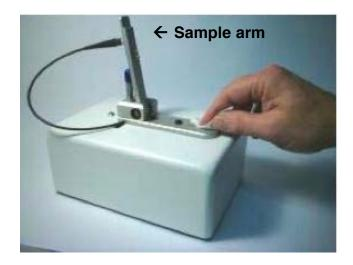
4. Pipette 2  $\mu$ l of ddH2O onto the measurement pedestal, as shown in the picture.
