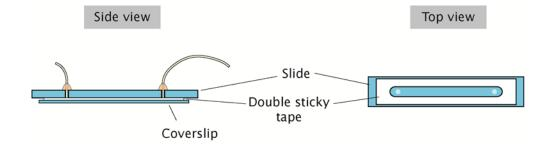
The chamber is made out of a microscope slide that has two holes drilled. Double sticky tape is sandwiched between this slide and a microscope coverslip. The tape is cut such that a little chamber is created between the coverslip and the slide. Tubing is connected to the holes using Epoxy.
