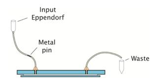
Liquid goes in by gravity. All you have to do to change the flow speed is to move the Eppendorf tube up and down! Be careful! If the tube goes below the chamber you'll get backflow! To stop the flow, put the input Eppendorf level with the slide.
