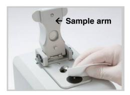
Pipette 2  $\mu$ l of "blank" buffer (in today's case, you would use 2  $\mu$ l of plain **Solution C6**) onto the measurement pedestal (as shown).
