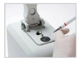
Gently lower the arm to the downward position and click the **Blank** button. During the measurement, the device will form a sample column between the two pedestals and adjust automatically for an optimal path length (0.05 mm - 1 mm).
